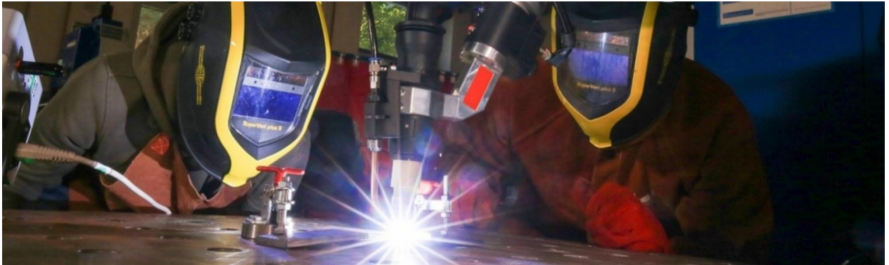
Metall-Aktivgasschweißen – MAG – mittels Cobot (Metal active gas welding – MAG – with cobot).
