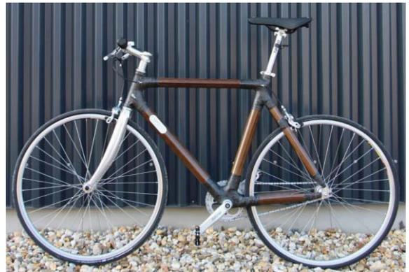
*Fahrrad aus Bambusrohren. (Bicycle made from bamboo.)*
